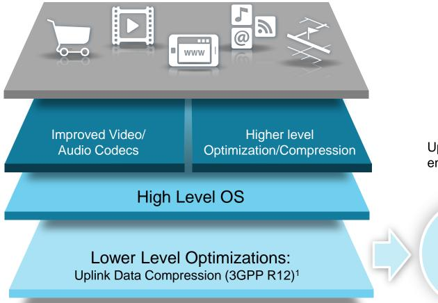
Uplink data compression is part of a group of 3GPP R12 uplink enhancements for improved coverage, capacity and load-balancing.
