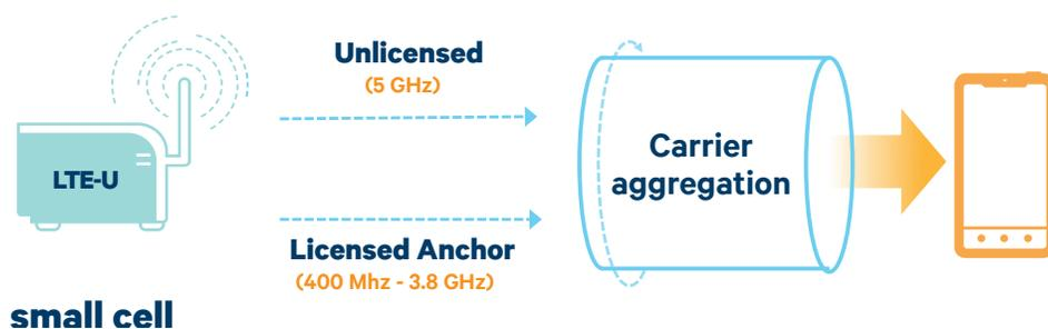
Fig. 6: LTE Unlicensed for new small cells
