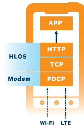
Fig. 5: Modem-level LTE – Wi-Fi link aggregation
