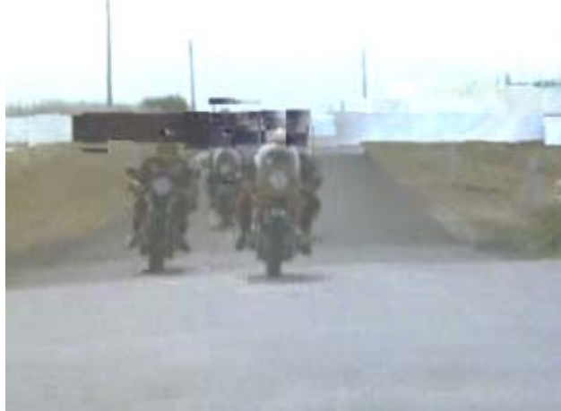
Figure 1. Example of the effect of minor packet loss on a video image.
