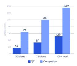
Figure 6.4 Latency (95th percentile, in milliseconds) for Qualcomm Technologies' OFDMA and competitor systems by traffic type scenario and background traffic load
