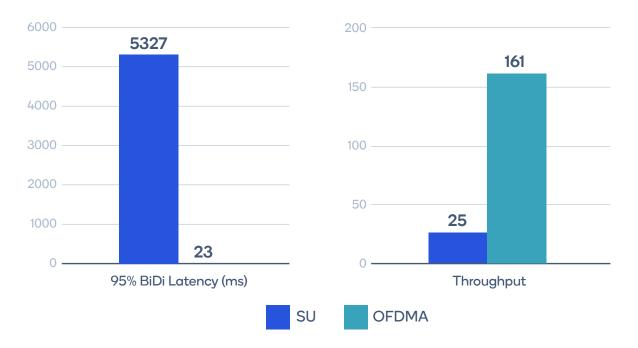
Figure 6.3 Impacts on latency (95th percentile, in milliseconds) and systems throughput (in Mbps) single user (SU) mode versus OFDMA with full buffer background traffic for a bi-directional gaming scenario and an uplink video scenario (AC\_VO)
