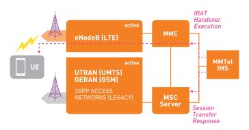
With acknowledgements that the commands have been executed, the user's device and the IMS/MMTel—still in control of the user's voice call in progress—switch to the CS network to continue the call. (Figure 8)
