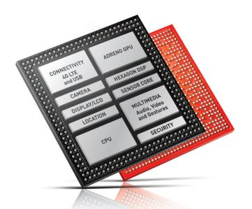
Snapdragon 600 series high-tier processors are designed to support a high-value combination of advanced features, superior performance, robust connectivity and all-day battery life in leading devices.
