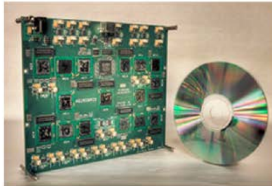
Real-time neuromorphic multi-chip emulator (NeuroGrid).
