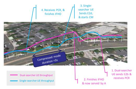
Figure 3: Part of drive route showing IFHO-related mobility events for Scenario 2 (Image generated using Google Earth TM)
