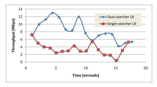
Figure 2: Throughput comparison during period where the two UEs have different serving NodeBs
