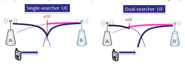
Figure 2: Scenario 1 – UE moving into the hotspot
