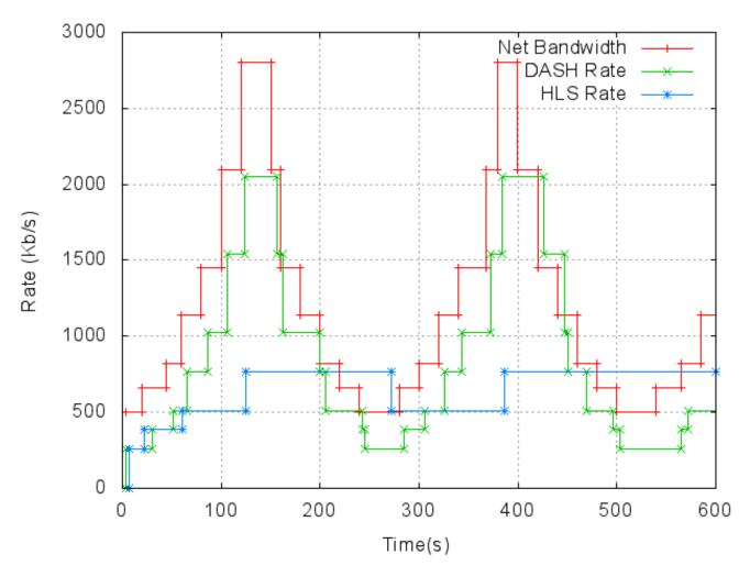
Figure 6 Qualcomm DASH client and HLS performance (controlled network case)
