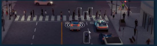
Vehicle-to-network e.g., real-time traffic/routing, cloud services.V2N messages enable valueadd use cases for drivers, vehicle OEMs and road operators Vehicle-to-pedestrian e.g., safety alerts to/from Vulnerable Road Users (VRUs) like bicyclists/pedestrians. Vehicles/VRUs broadcast messages on a sidelink channel allowing other actors to take appropriate action
