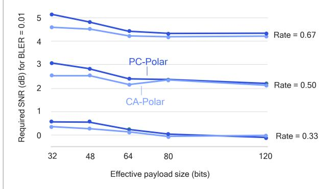
1. Parity-Check Polar channel coding
