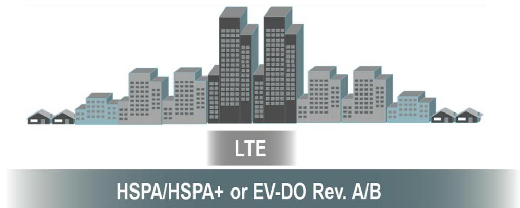
*Figure 2: LTE overlay on a 3G network*
