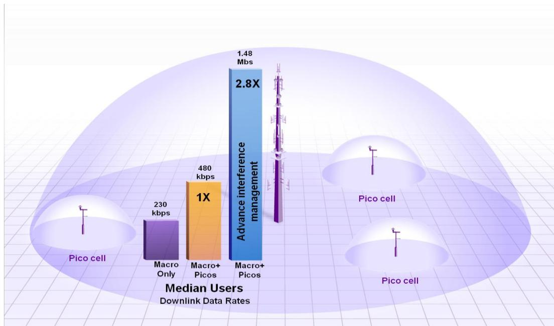
Note: Assuming 10 Picos per macro randomly dropped within macro coverage. Preliminary results based on simplified set of simulations and some advanced interference management techniques. Based on proposed LTE-A evaluation methodology in R1-08402610 MHz FDD, 2x2 MIMO
