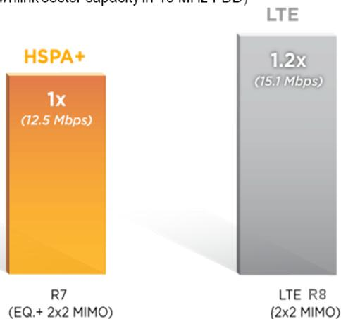
Note: Handset Interference Cancellation and HSPA+ multicarrier MIMO would further improve HSPA+ spectral efficiency.
