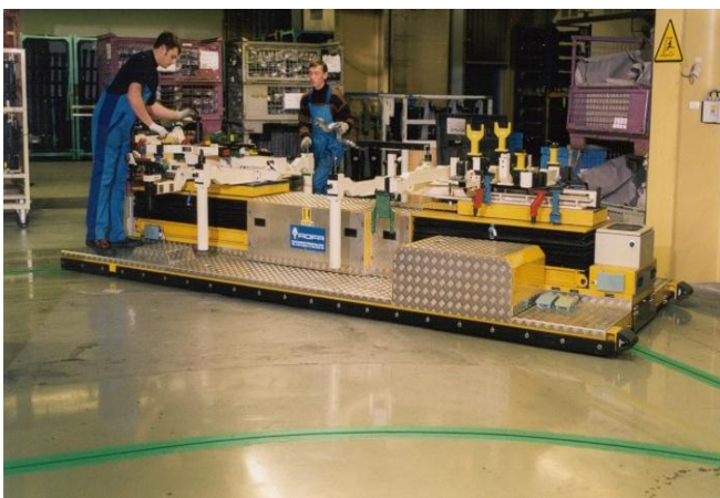
(b)Figure 1b: An AGV system powered using IPT, with vehicles electronically guided to follow a magnetic path.
