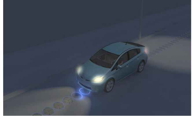
Figure 5: A Possible IPT Powered Highway (a) Pads buried in the road supplied by roadside cabinets (b) Only pads under the vehicle are energised
