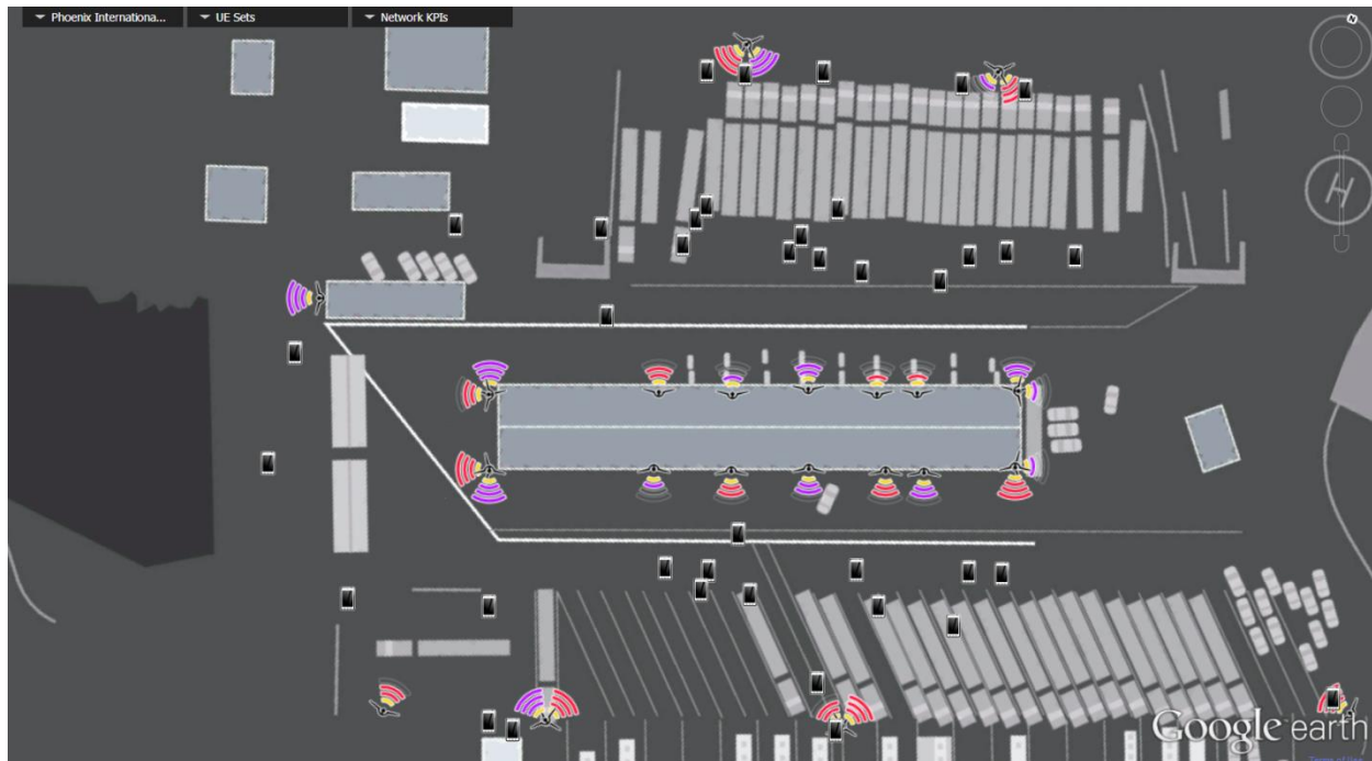
Figure 11: Network configuration and UE placement, as used during the capacity testing
