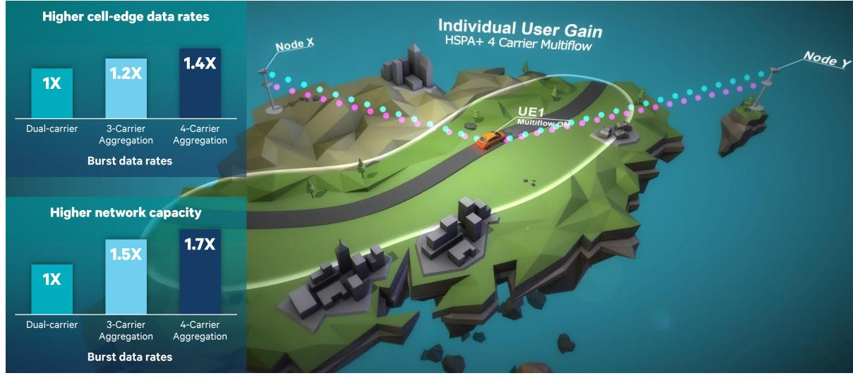
Assumptions: 57 cell wrap around with 1km Inter-site distance (ISD). Receiver type LMMSE, Rx Diversity. Traffic model: 3GPP bursty source with 1 Mb burst, exponential inter-arrival with 5s mean. Power allocation: 30% total overhead power (incl. 10% of C-PICH). Antenna pattern: 2D with 70deg 3dB beam width. Channel Model: PA3. HS-DPCCH Decoding: For Intra-NB, at Node-B with soft combining. For inter-NB, at both NodeBs.
