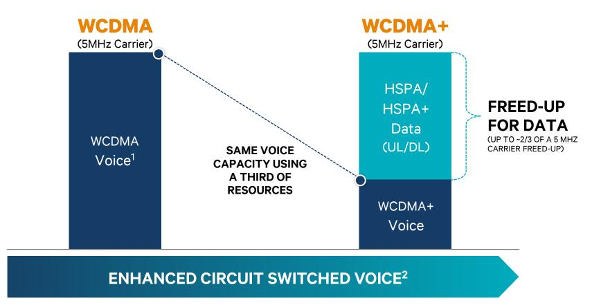
There is ~10% DL data capacity available at max voice capacity not shown in the graph for WCDMA .Assumptions: single receive antenna and rake receiver assumed for voice, dual receive diversity assumed for data.
