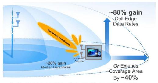
Source: Qualcomm simulation for closed loop beamforming 3GPP framework PA3, 4UEs per cell, 2.8km ISD. Shows data throughput gain for the median and the 59 worst. (Cell edge) users. Gain depends on propagation environment and the UE speed with lover gain for faster moving users.
