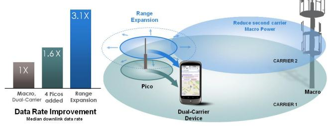
4 Picos added per macro and 50 % of users dropped in clusters closer to picos (within 40m), Model PA3 full buffer ISD 500m. Enabling range expansion features: reduced power on second macro carrier, dual carrier devices and mitigating uplink and downlink imbalance (3dB Cell-individual offset (CIO) and pico noise-figure pad)
