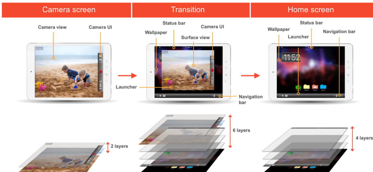
Figure 12: Compositing multiple UI layers for a transition from camera to home screen
