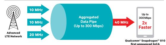
LTE Advanced device simultaneously receives on three radio channels which increases user data rates and reduces latency (faster network response time) as compared to conventional LTE devices
