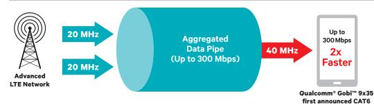
LTE Advanced device simultaneously receives on two radio channels which increases user data rates and reduces latency (faster network response time) as compared to conventional LTE devices
