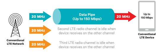
LTE device receives only on one radio channel with maximum data speed limited by radio channel bandwidth
