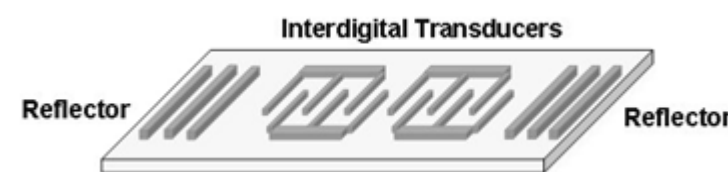
Figure 5: Schematic diagram of a SAW component
