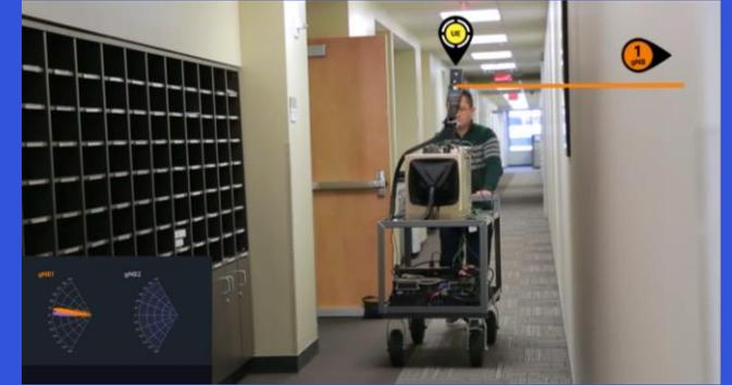
Demonstrating sustained mobile communications indoors, with wall penetration and hand/body-blocking
