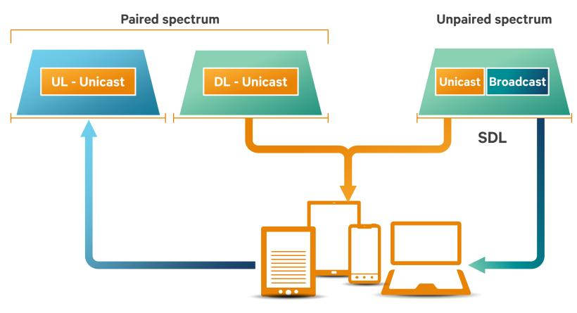
Better utilizing unpaired spectrum for downlink intensive traffic
