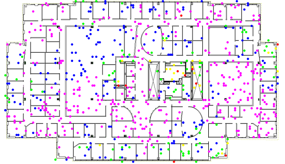
Fig. 6. Received power map of 29GHz when only AP 1 is active.
