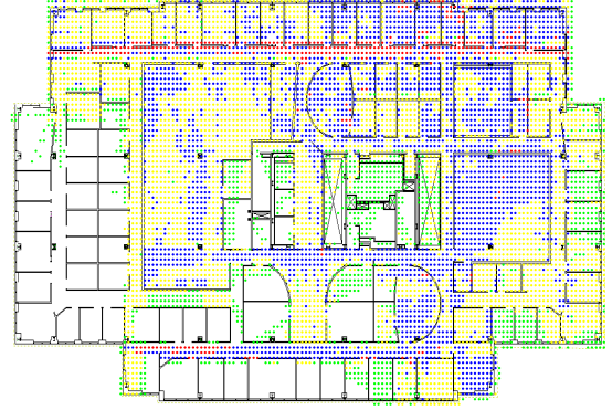
Fig. 9. Map of the number of clusters seen by a receiver in the vicinity of access point 1. Green: 1 or 2, yellow: between 3 and 7, blue: between 8 and 12, and red: 13 or more beams. White space = no detectable beams.
