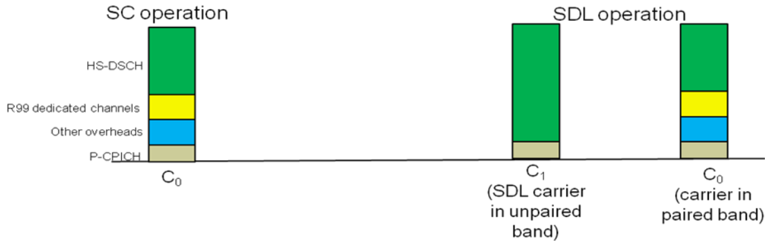
Figure 2: Power per channel differences between Single Carrier and SDL operation
