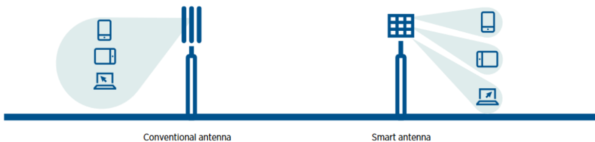
Figure 2: Conventional antenna coverage compared to the antenna with beamforming
