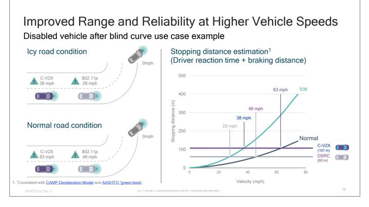
The intent of these simulation plots is to signify the advantage of vehicles operating with C-V2X compared with DSRC in real life conditions.
