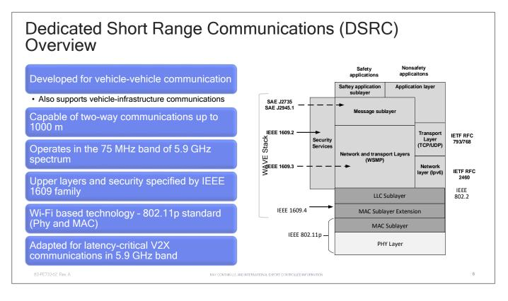
DSRC or Dedicated short range communication is a type of V2X technology which provides the ability for vehicles to communicate with other vehicles and infrastructure around them, exchanging BSMs (Basic Safety Messages) for collision avoidance.
