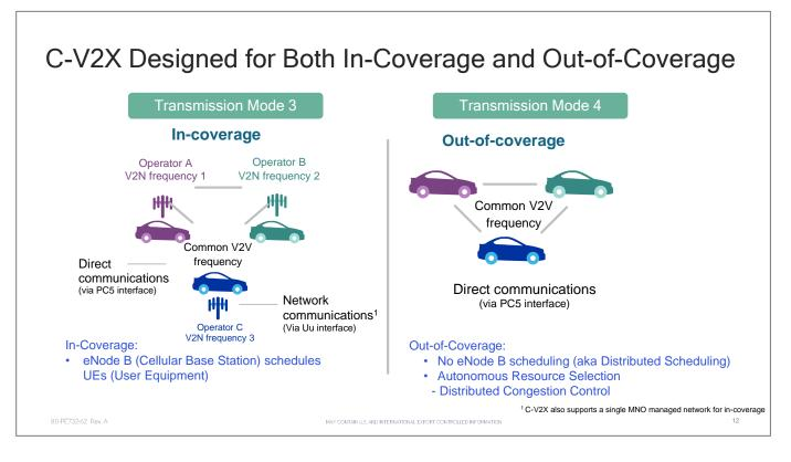
C-V2X designed for both In-coverage and Out-of-coverage.
