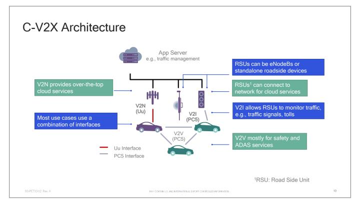
Cellular-V2X defines a new air interface called PC5 for V2V, V2I communication. V2N is still over the legacy LTE Uu air interface and provides over the top cloud services.
