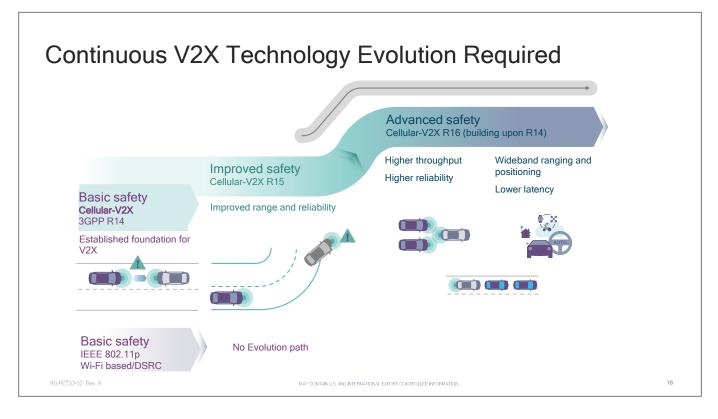
3GPP Release 14 based C-V2X establishes the foundation for V2X communication for basic safety messages exchange.
