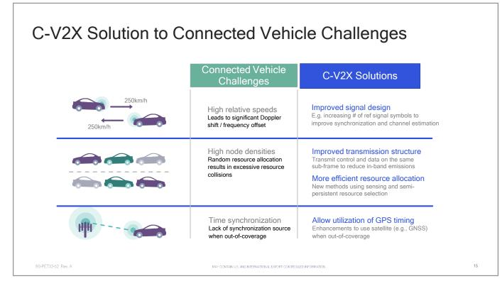
Vehicles at high speeds face a challenging RF environment for message transmission and reception.
