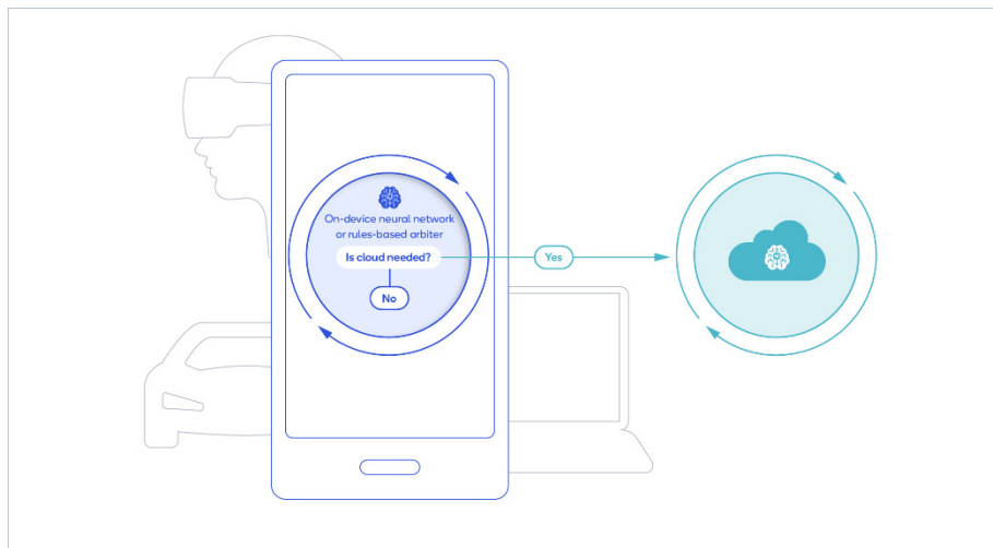
Figure 2: In a device-centric hybrid AI architecture, the cloud is only used to offload AI tasks that the device cannot sufficiently perform.
