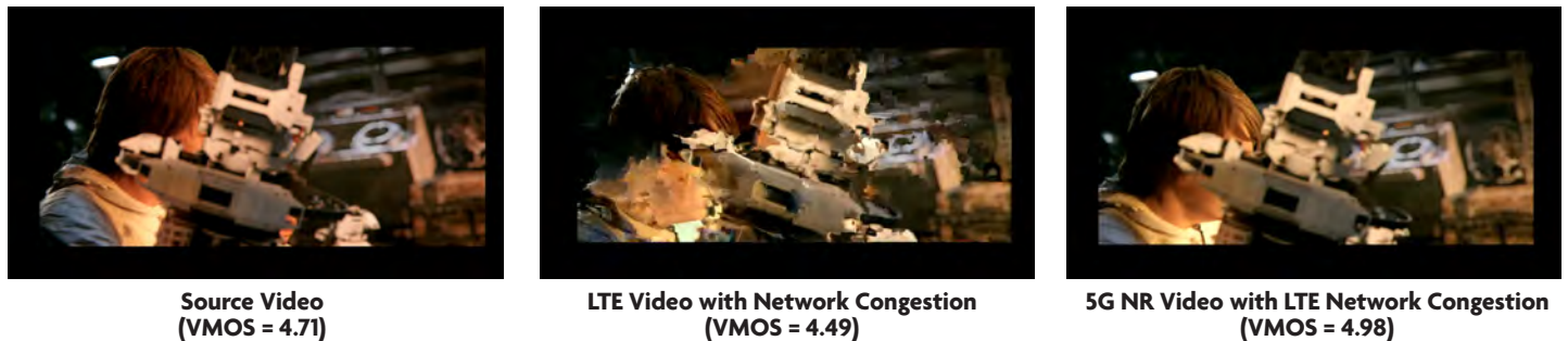
Figure 31. Source Video versus LTE Loaded Video versus 5G NR + LTE Video, II
