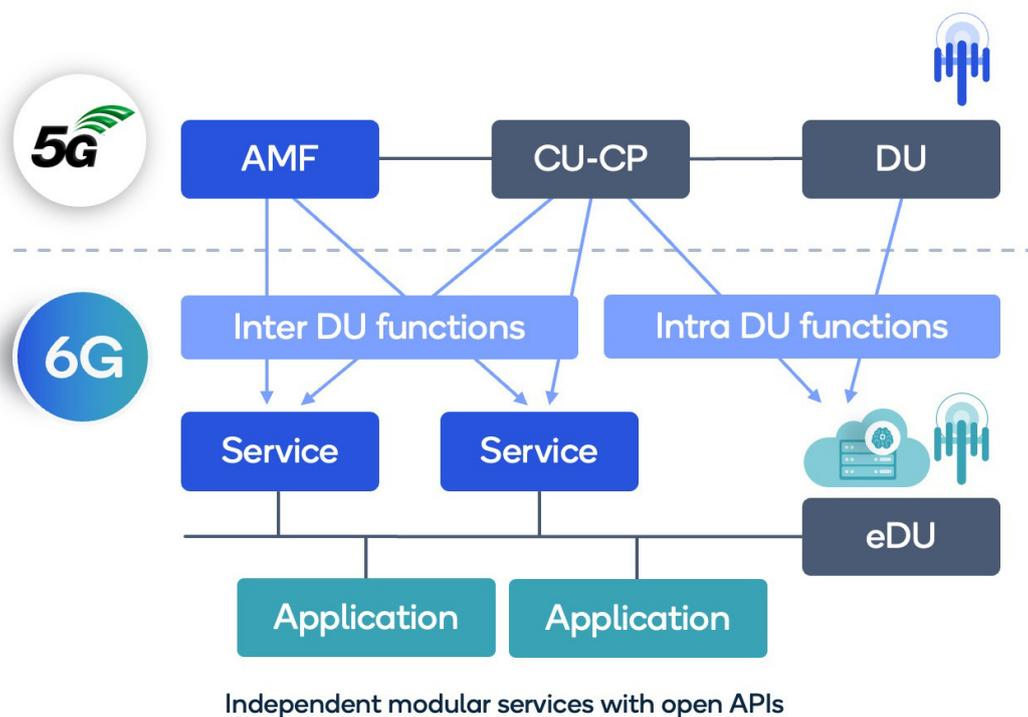
**Figure 23: Functional split from 5G to 6G, with vertical convergence and horizontal split**
