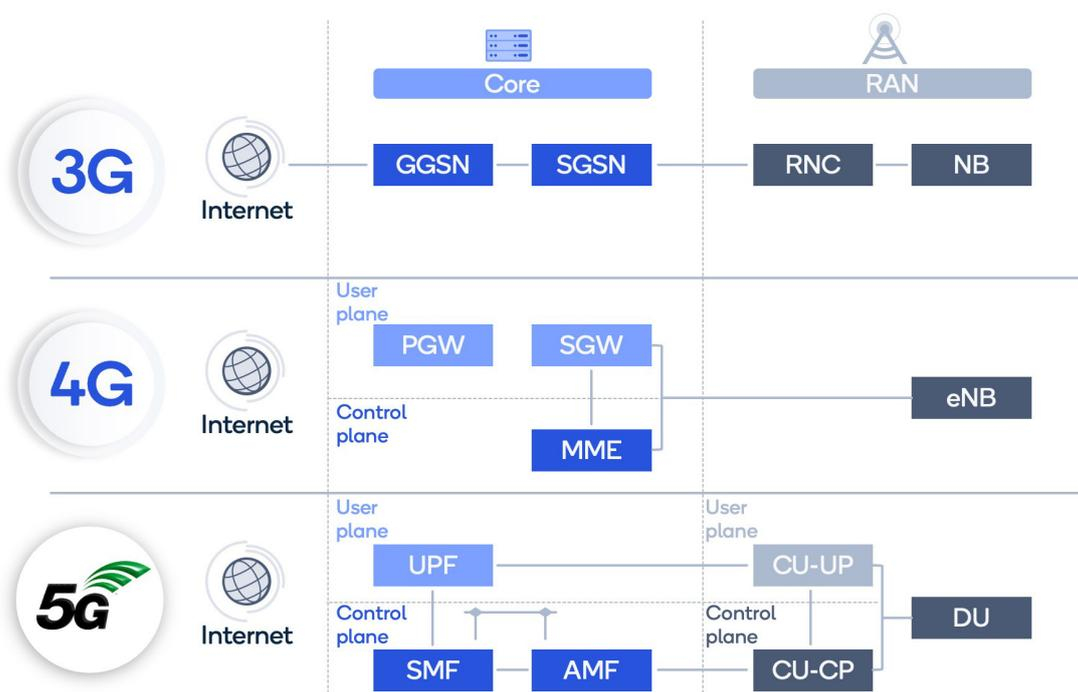
Figure 21: Increasing disaggregation of network from 3G to 5G
