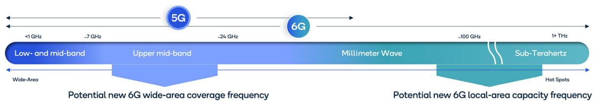
Figure 27: 6G is expected to improve utilization of existing bands and expand into new bands
