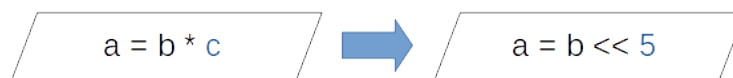
Figure 3-4 Downgrading ALU instructions (assuming c is calculated as 32 and invariant during the kernel execution)
