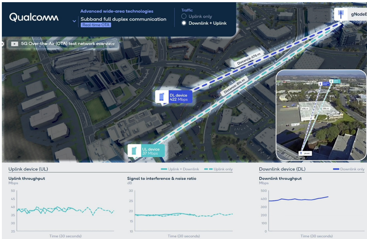
Figure 3. Over-the-air performance of subband full duplex in 3.5 GHz
