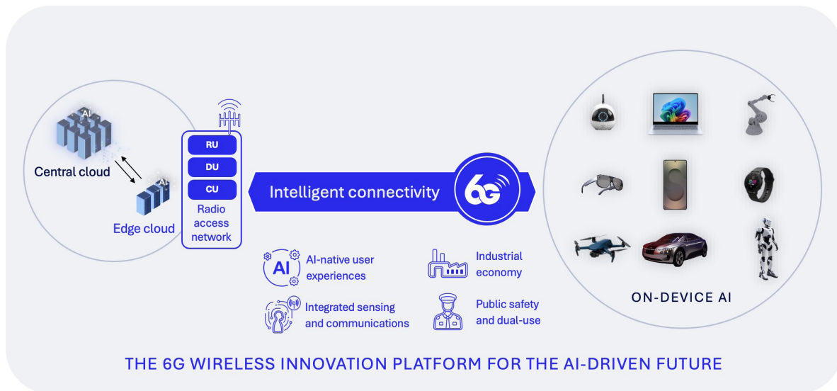
Figure 5. The hybrid AI architecture spans the device, edge and cloud
