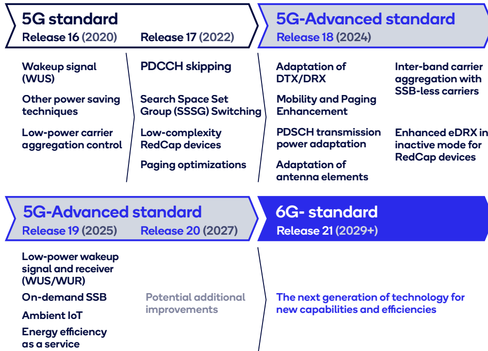
Figure 6. The 3GPP has consistently pursued energy efficiency improvements for 5G and 5G-Advanced networks
