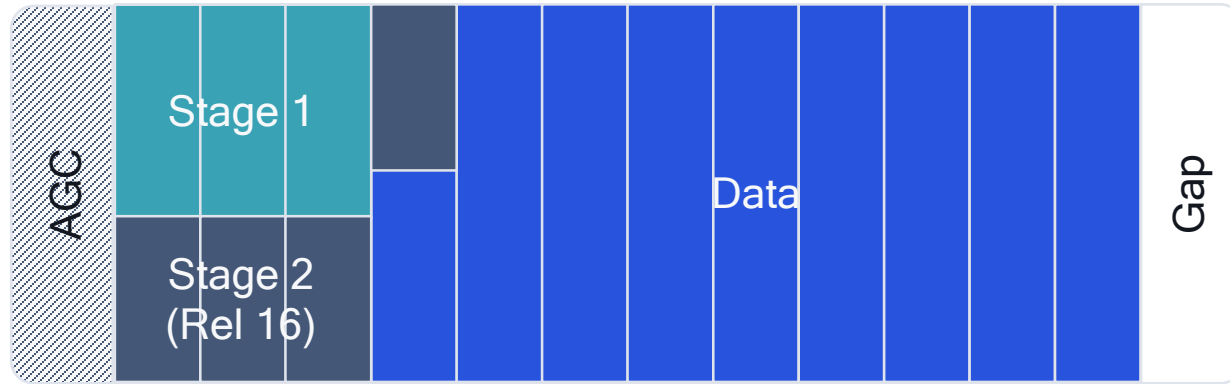
Slot structure showing two-stage control
