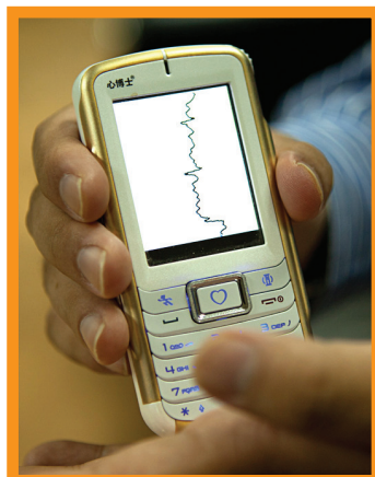
A patient uses the 3G cardiovascular sensing device to measure his heart data, which will be sent to a specialist for feedback in real-time.
