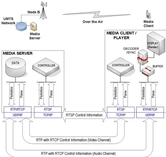
Figure 1 Typical VS Protocol Architecture
