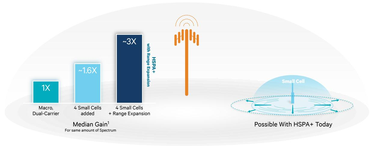
Gain in median downlink data rate, 4 small cells of pico type added per macro and 50 % of users dropped in clusters closer to picos (within 40m), Model PA3 full buffer ISD 500m. Enabling range expansion features: reduced power on second macro carrier, Dual-Carrier devices and mitigating uplink and downlink imbalance (3dB Cell-individual offset (CIO) and pico noise-figure pad)
