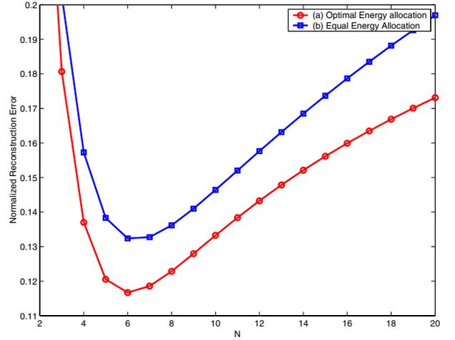
Fig. 8. With  $\sigma_k^2 = 0.01 \times k, \forall k$  and,  $\{d_1, d_2, \dots, d_{10}\} = \{1, 5, 1, 5, 1, 1, 5, 5, 1, 5\}$ : (a) Normalized value of the objective function in (20) with optimal energy allocation among sensors. (b) Normalized value of the objective function in (20) with equal energy allocation among sensors.
