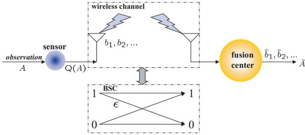
Fig. 1. System model of a single sensor's quantized measurement received through a BSC at the fusion center.
