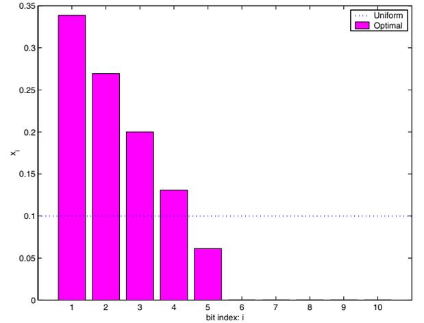
Fig. 4. Optimal energy allocation over a fixed number of quantization bits ( $N = 10$ ).
