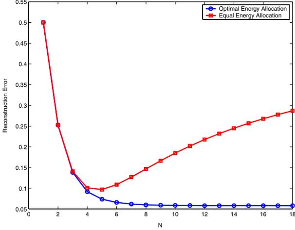
Fig. 5. Comparison between equal energy allocation and optimal energy allocation.
