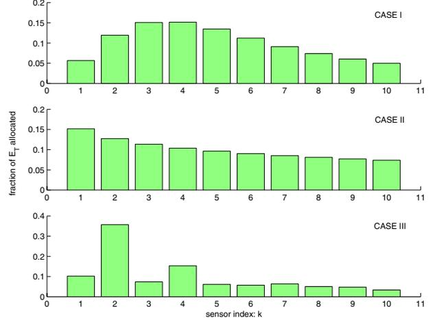
Fig. 7. Optimal energy allocation scheme when using the corresponding optimal number of quantization bits:  $N_{opt}$ . CASE I.  $d_k = k, \sigma_k^2 = 0.01, \forall k$ . CASE II.  $d_k = 1, \sigma_k^2 = 0.01 \times k, \forall k$ . CASE III.  $\sigma_k^2 = 0.01 \times k, \forall k$  and,  $\{d_1, d_2, \dots, d_{10}\} = \{1, 5, 1, 5, 1, 1, 5, 5, 1, 5\}$ .
