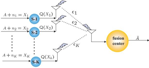
Fig. 2. Multi-sensor cooperation in estimating a scalar parameter with quantized observations.
