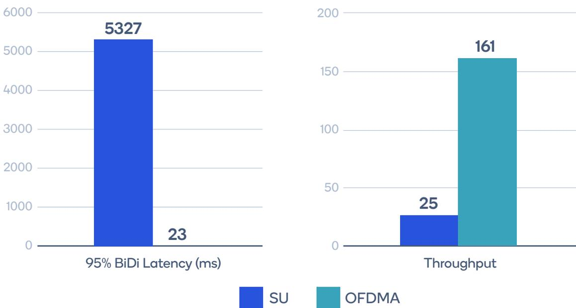
Figure 6.3 Impacts on latency (95th percentile, in milliseconds) and systems throughput (in Mbps) single user (SU) mode versus OFDMA with full buffer background traffic for a bi-directional gaming scenario and an uplink video scenario (AC\_VO)
