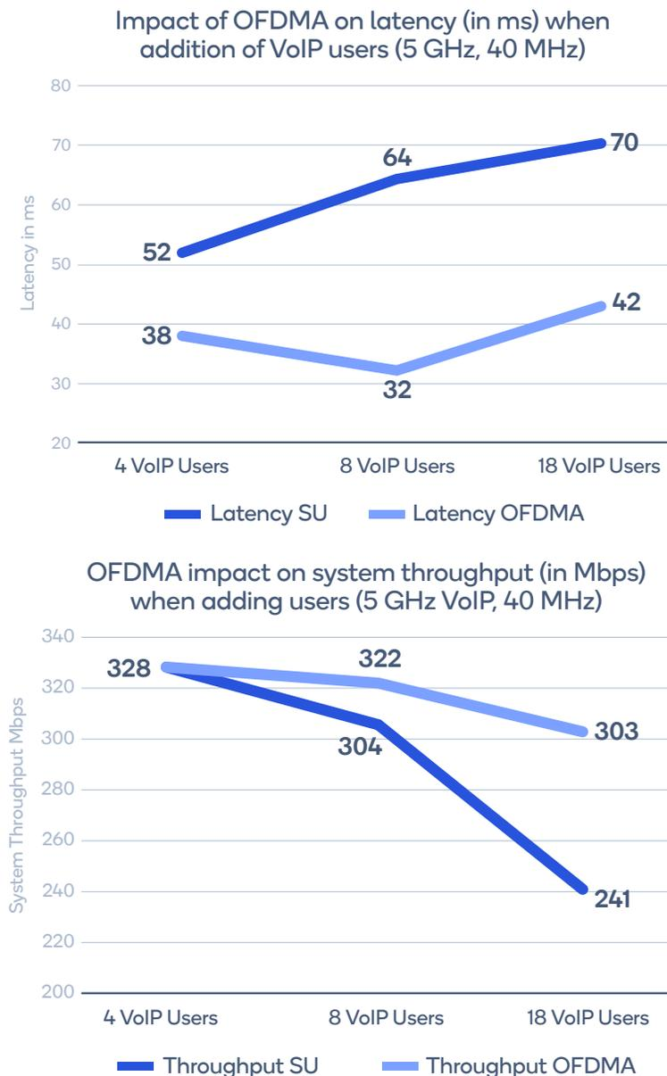
Figure 6.2 Impacts on latency (95th percentile, in milliseconds) and systems throughput (in Mbps) of 4, 8, and 18 VoIP users, single user (SU) mode versus OFDMA with full buffer background traffic
